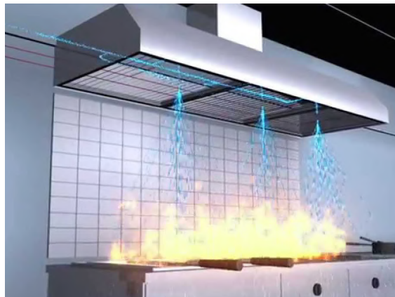
Kitchen fire suppression
